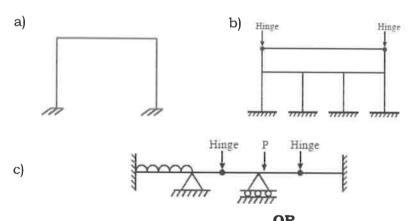
Find the Static Indeterminacy and Kinematic Indeterminacy for the Q.2(B)10M 5 following Pin Jointed Frames.
