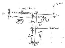
Q.5(A) Analyze the Continuous beam ABCD loaded as shown in Fig. by 10M 4 5 Moment Distribution Method. Sketch the bending moment diagrams.
