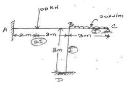
**Q.6(A)** Analyze the Continuous beam ABCD loaded as shown in Fig. by 10M 5 5 Kani's Method. Sketch the bending moment diagrams.
